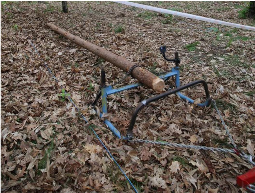
**Figure 2.** Use of the sled during the trials, with the front part of the log resting on the sled, greatly reducing the area of contact with the ground. The sled is a simple system, easy to manufacture, and is attached to the swingle tree via a “V” shape chain, in the front part.
