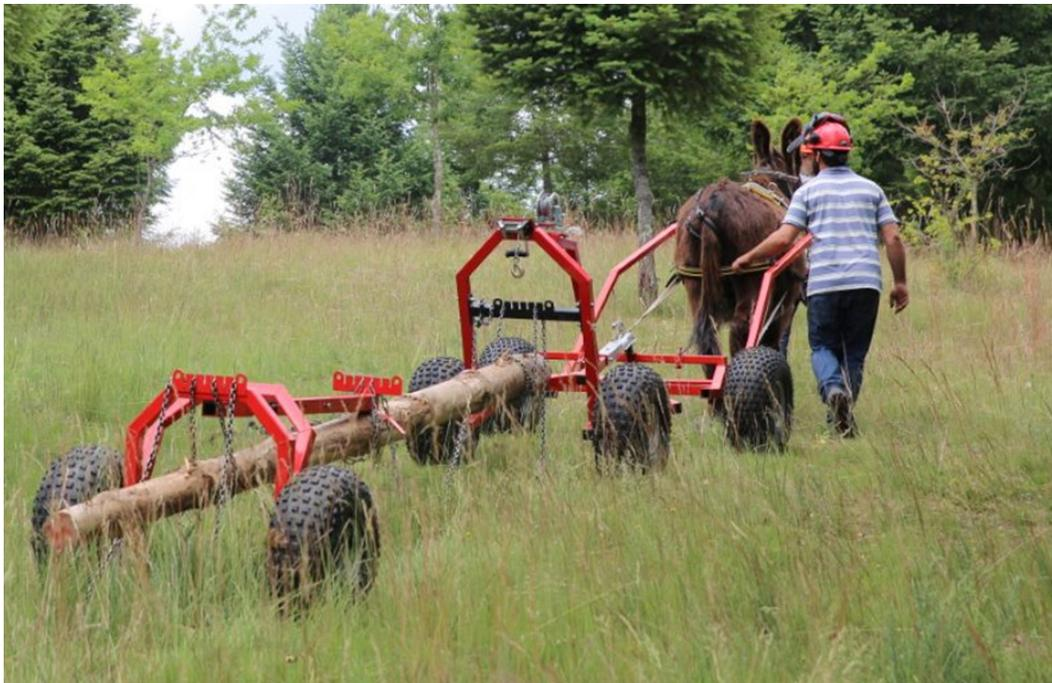
**Figure 3.** Vehicles in use while carrying the 0.1 m<sup>3</sup> log. Note that 2 logging arches keep the log fully suspended (rear and front logs). The front log is then attached to the forecart via a tow ball. Note the complete cart harness in place, using a breeching and a cart saddle.
