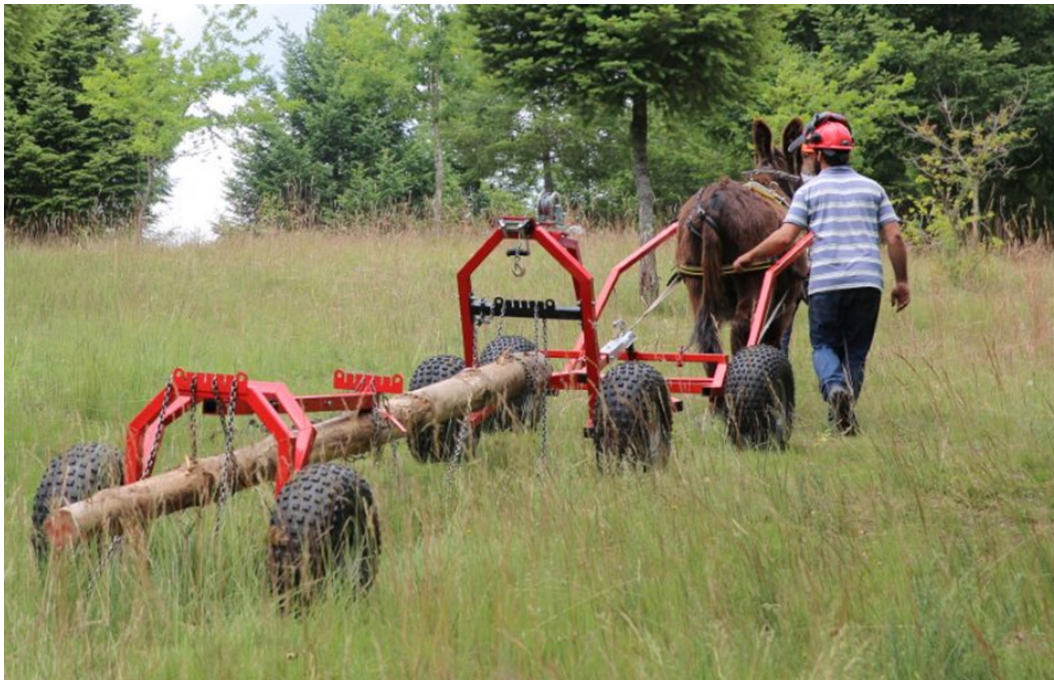
Figure 3. Vehicles in use while carrying the 0.1 m 3 log. Note that 2 logging arches keep the log fully suspended (rear and front logs). The front log is then attached to the forecart via a tow ball. Note the complete cart harness in place, using a breeching and a cart saddle.
