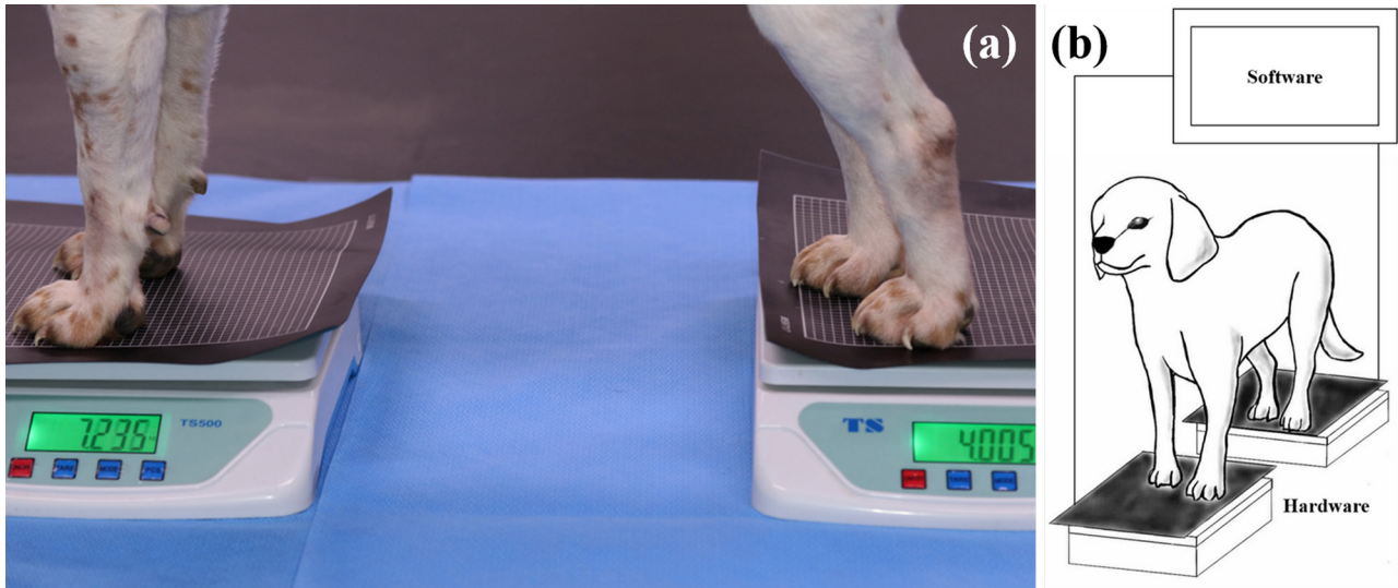
Figure 2. Placement of the dog and devices during measurement (a). As a simplified schematic for measurement, the software was created using the PetLAB2 program, and the hardware is composed of a digital weighing scale, force-sensitive resistor, and data acquisition electronics (b).
